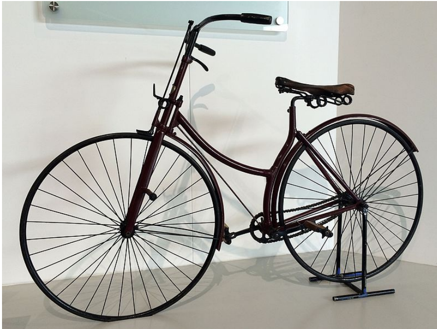
The 1886 Rover "safety bicycle" (with permission of British Motor Museum).
