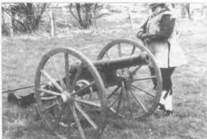
Minion, a slightly larger calibre gun weighing 1,200 lbs 3¼" calibre, wt of shot 3¼lbs
