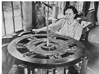
A mahogany braiding machine at G & J Zair, whip makers, constructed to the design of George Dundass
